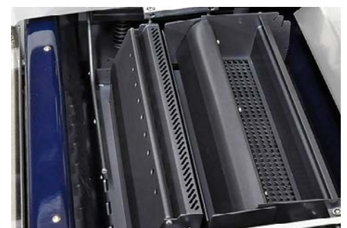
Solder module with pre-solder and finishing nozzle
