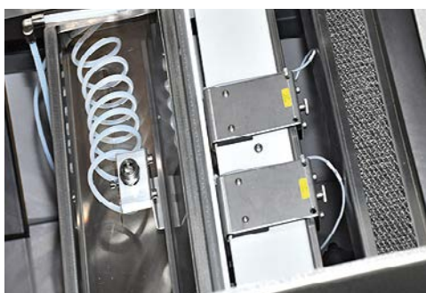
Precision spray fluxer (optional) with blow off device
