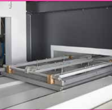
Optional automation solution with view on the transfer of the carrier from the lifting station to the conveyor belt.
