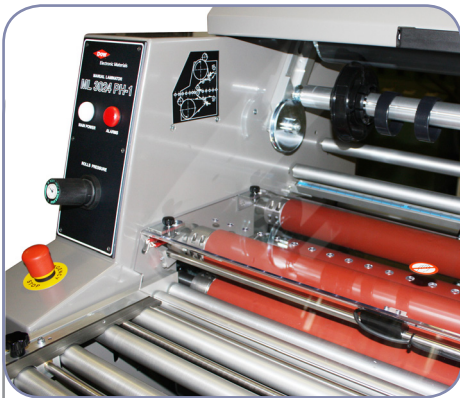
Pre-Heating section made by two hot rolls
