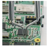
Hand soldering with the Chip Tool for the smallest SMT chips
