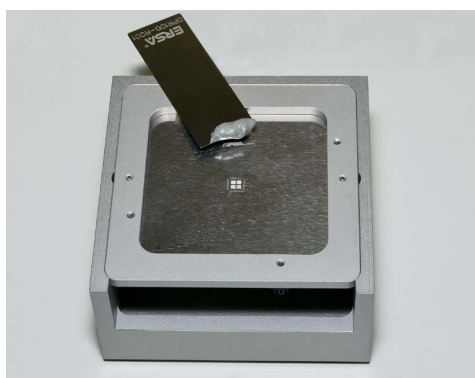
Dip & Print Station with "MLF32" stencil
